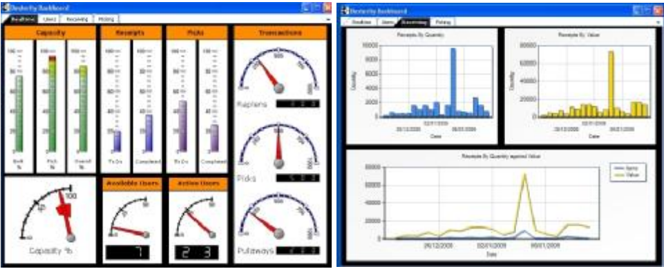
"Real Time" views of Receipts, Picks, User Activity & Warehouse Capacity Graphical representations of any warehouse data including pick activity &
